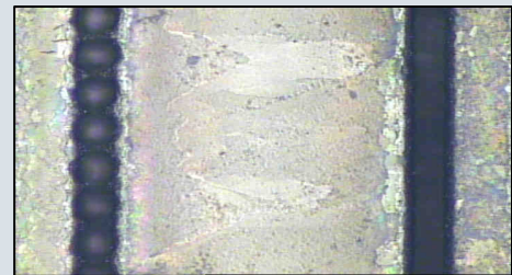
Left: Gaussian Grooves in TCO-Layer. Right: Top-Hat Grooves in TCO-Layer. Laser: Nd:YAG, SHG @532nm, 4W, 500kHz, 10ps-pulses
