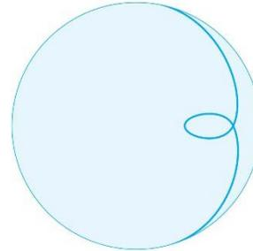
Adjust either the laser rod or the alignment beam to make these loops and cusps disappear. Now the alignment beam accurately follows the optical centerline of the laser rod. There may be limiting apertures that prevent the laser beams from striking the edges of the laser rod. In that case adjust the alignment beam and rod to make the beam pass through the center of the apertures.
