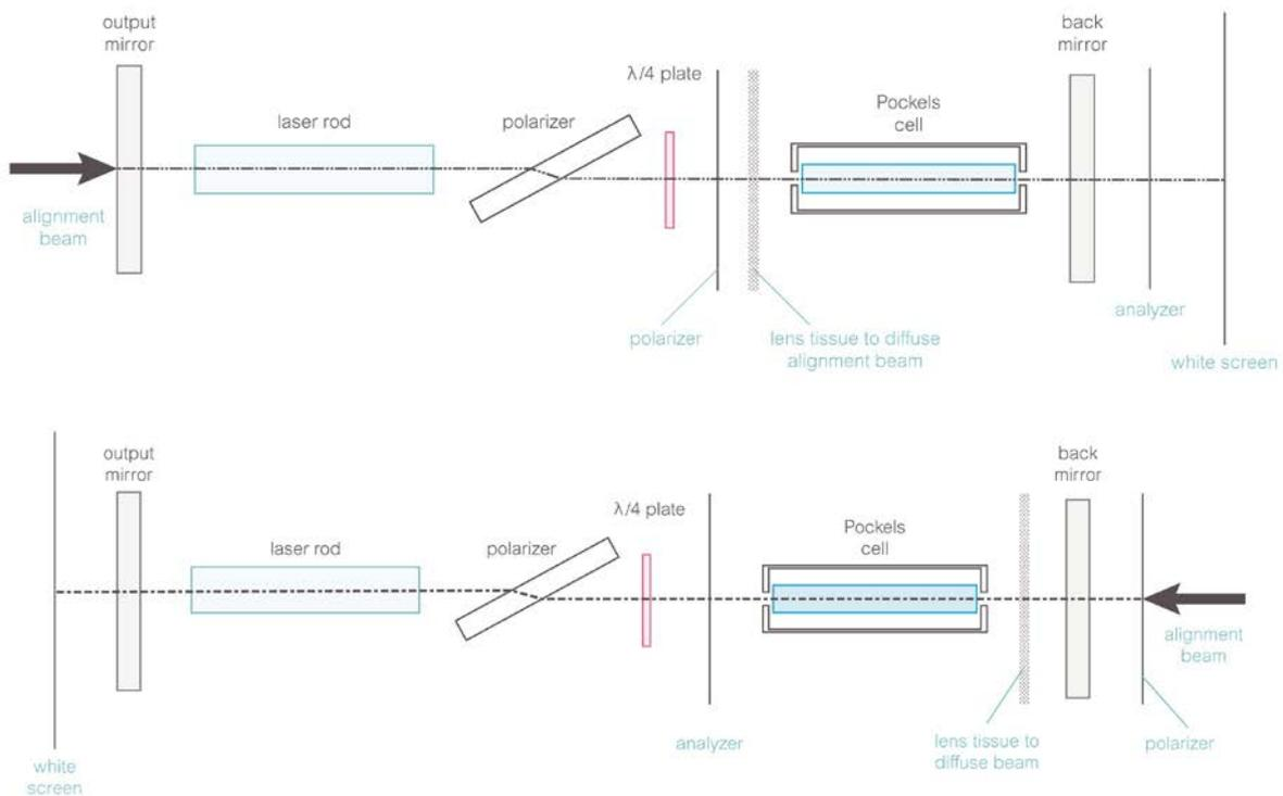
Schematic illustration of a typical Q-switched laser system with components added for Pockels cell alignment.
